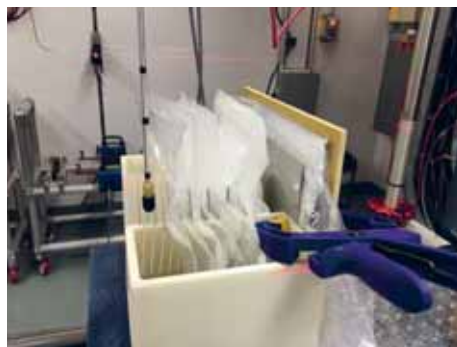
Figure 1: Experimental setup for measuring the dose reduction after a multilayer configuration with a proportional EGG counter.
