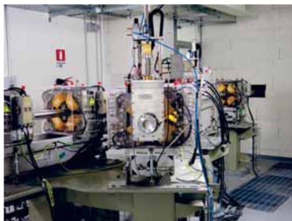
Figure 2: A detail of the 30° beam line exit window. The vacuum in the beam pipe is maintained by a 70 \mu\text{m} thickness titanium layer. A beam profile monitor is also present just before the exit window.
