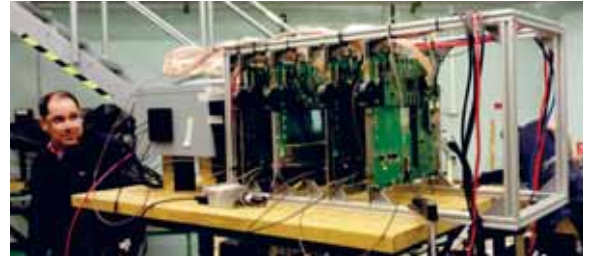
Figure 1: pCT apparatus at The Svedberg Laboratory (Uppsala, Sweden) beam line : tracker (green boards) and calorimeter(gray box).
