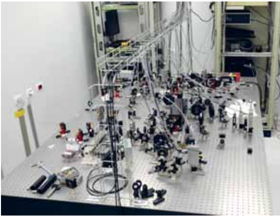
Figure 2: Squeezed states of light are used to beat quantum noise in gravitational wave detectors. Picture of the squeezed light source under development at Advanced Virgo, European Gravitational Observatory, Pisa.
