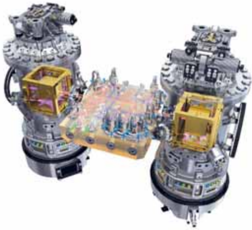
Figure 1: Key LPF hardware, including the Gravitational Reference Sensor (GRS): 2 kg Au-Pt test masses inside the electrode housings (gold); UV discharge illumination (purple); (surrounding) vacuum chamber and TM caging hardware.
