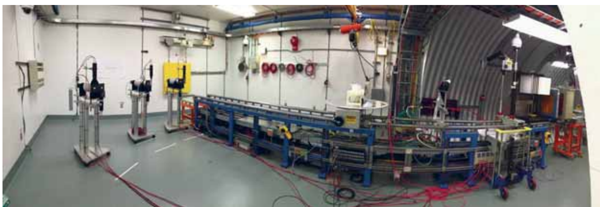
Figure 2: Experimental setup for measuring secondary neutron yield after a lithium hydride sample. A set of three telescope composed of a thin plastic scintillator and a liquid scintillator are placed at several angles with the respect to the primary beam direction at a distance of 3 m from the target. Energy deposition and time-of-flight (TOF) of secondary neutrons emerging from the target are acquired to obtain their yield and kinetic energy spectra.
