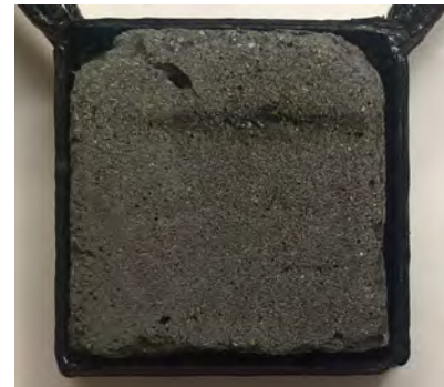
Figure 4: The asteroid simulant material, the darker horizontal line denotes the ablated region.
