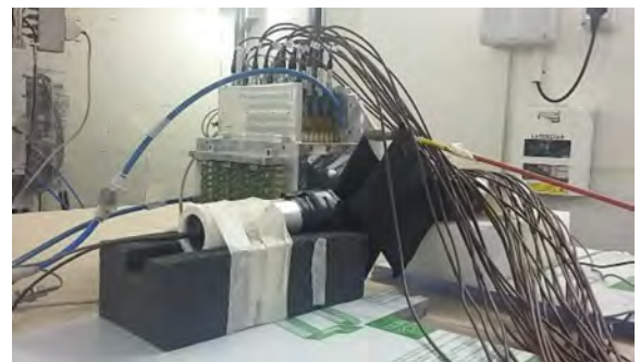
Figure 1: Drift Chamber and plastic scintillators used at the Trento Proton Therapy center for the experiment.
