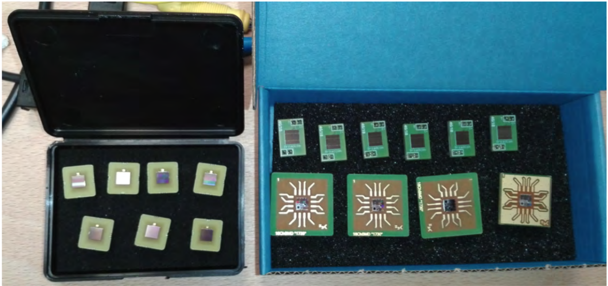
Figure 8: FBK-AVANSID SiPMs before irradiation. All samples are I - V characterised after irradiation. Several samples are mounted on PCB for studies of radiation damage at pixel level (blue box on the left).
