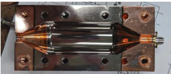
Figure 1: One of the two halves of the superconducting cavity. The cylindrical body is 50 mm long with diameter 26.1 mm, while the cones are 19.5 mm long.
