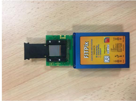
Figure 1: *Fitpix* chip connected with the hybrid 3D Silicon neutron detector (not filled with *LiF*).
