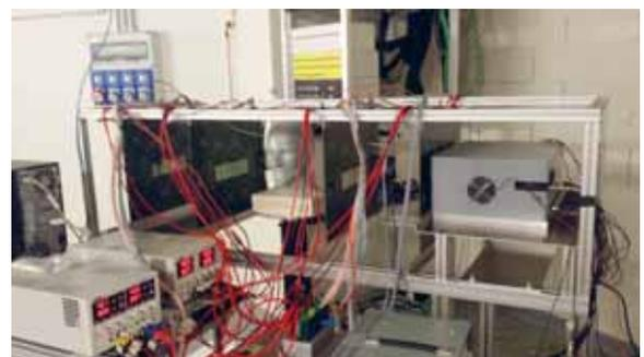
Figure 1: The Prima-RDH-IRPT pCT system mounted on the Trento Proton Therapy center experimental beam line. The four tracker planes (green boards), the anthropomorphic phantom and the calorimeter (inside the grey box) are visible. The proton beam enters the apparatus from left.
