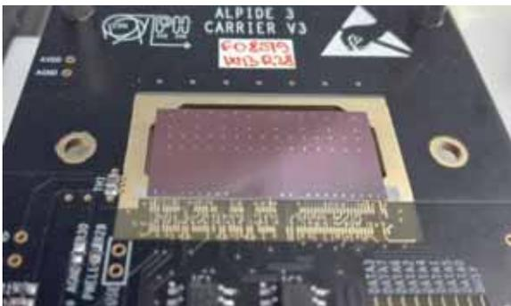
Figure 4: The ALPIDE sensor on the carrier board.
