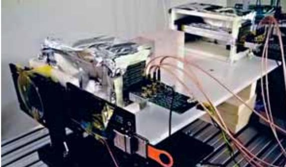
Figure 3: Experimental setup installed at the TIFPA irradiation facility. The tracker ALPIDE sensor sits in the leftmost instalment, followed by the first calorimeter station with the one-plane front-end electronic visible. After the plastic absorber, the second calorimeter station is visible. Both the calorimeter stations and the plastic absorber were arranged in different positions during testing.
