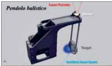
Figure 10: The aluminum target mounted on the ballistic pendulum in the KrF laser beam. The angular deflection of the Al target is obtained from the displacement of a second, reflected laser beam, in the vertical direction.
