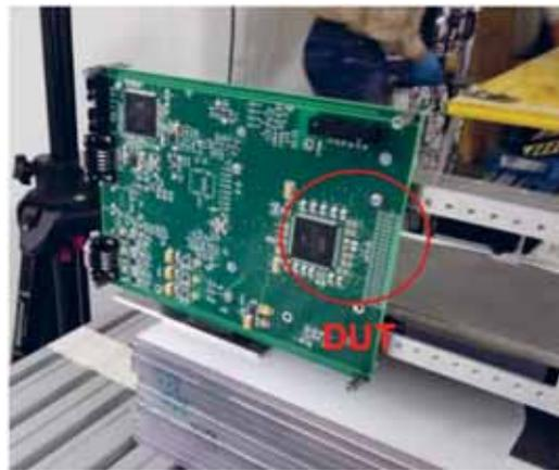
Figure 2: Test Board mounted on the XY translation stage.
