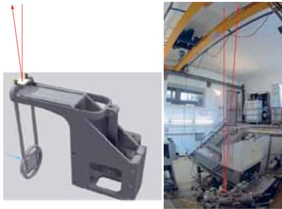
Figure 2: The Al target mounted on the ballistic pendulum in the KrF laser beam, blue arrow (left). View of the PLD laboratory, the angular deflection of the target is obtained from the displacement of a second, reflected laser beam, in the vertical direction, red arrows (right).
