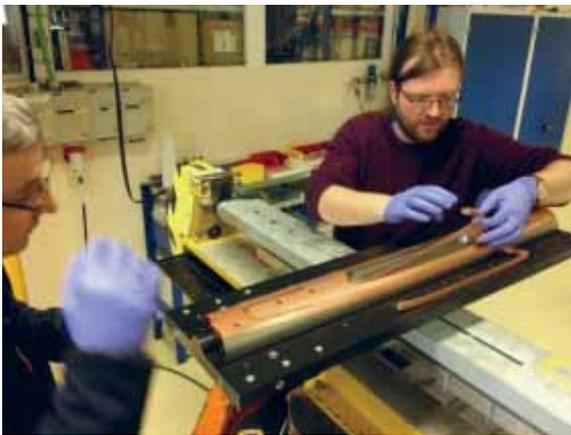
Figure 7: High luminosity LHC dipole test at CERN. Courtesy of Dr. G. De Rijk.
