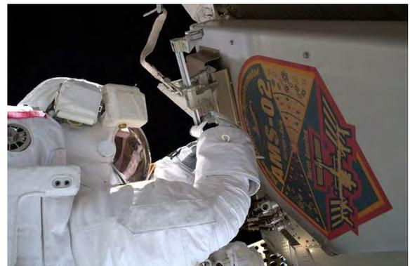
Figure 2: L. Parmitano concluding the UTTPS replacement for AMS on 25/01/2020. The spacewalk was completed in 5 hours and 58 minutes.
