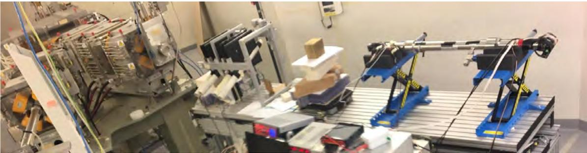
Figure 4: The HeCal prototype at the Trento proton beam line (70-240 MeV).
