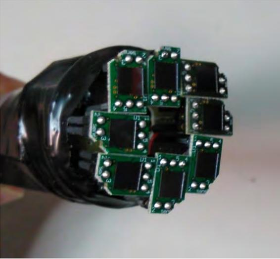
Figure 3: 8xSiPM ring array developed at TIFPA to replace the front PMT. The particles can enter in the HeCal detector avoiding to cross the sensitive photodetector surface.
