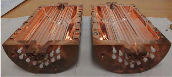
Figure 1: The two halves of the copper cavity complete of sapphire rods.
