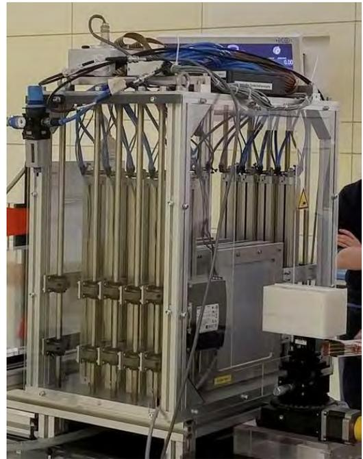
Figure 2: Customized binary range shifter developed for the high resolution microdosimetry and radiobiology measurements with the TIFPA proton beam, planned in the next year of the project.
