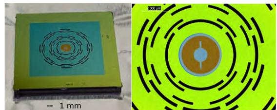
Figure 3: The TiN floating electrode on a  $\text{Si}_4\text{N}_3$  membrane. (left) the whole device (right) detailed region of the electrode (optical microscope image).
