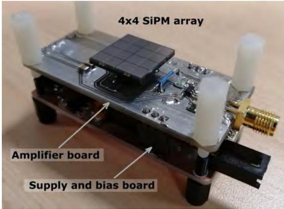
Figure 1: Assembly of SiPM detector, amplifier and bias/supply board
