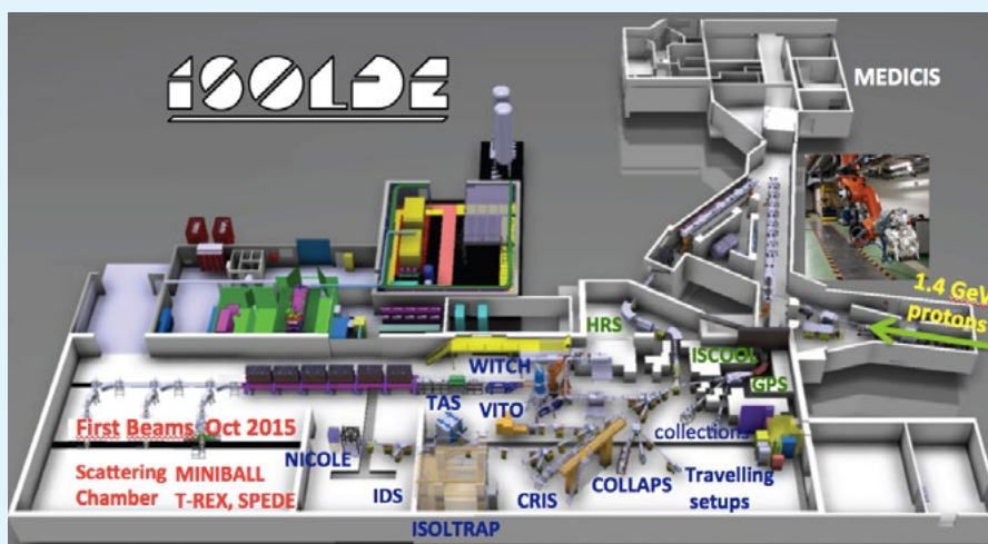
Schematic layout of the ISOLDE Facility, Switzerland. The different parts of the Facility and experiments are indicated: the two target stations connected to the mass separators of low resolution, GPS and higher resolution, HRS.
