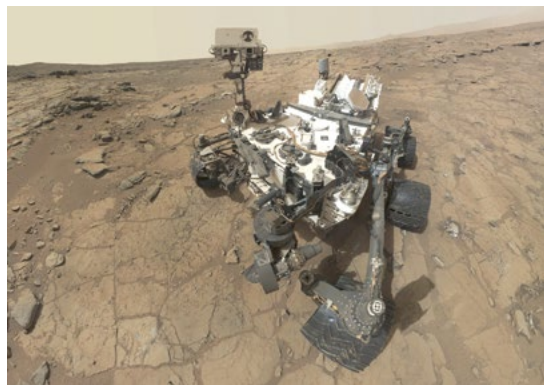
Figure 4: The NASA Mars Science Laboratory (MSL) spacecraft had onboard the Curiosity and a radiation detector (RAD), which has been used to measure the dose in deep space during the transfer to Mars (November 2011-August 2012) and on the planet's surface (photo courtesy of NASA)
